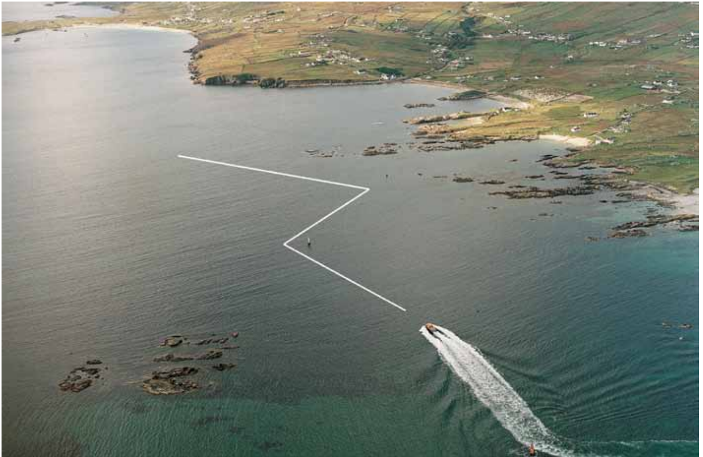
Arranmore lifeboat heading W from Aileen Reef towards Chapel Sound. The lifeboat has left Aileen Reef beacon (bottom R) close to port and is heading for Leac na bhFear beacon (centre). Aphort beacon is just visible above and to the right of Leac na bhFear. Rossillion Bay (Aphort) top L
